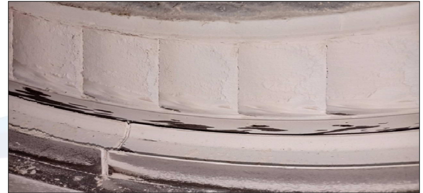
Silica formed on the nozzles
