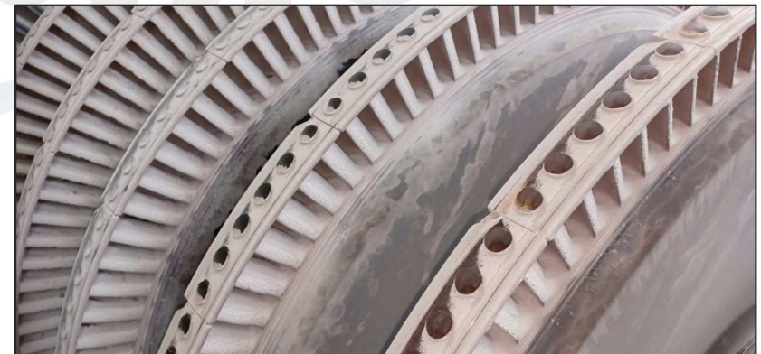
Silica formed on the moving blades
